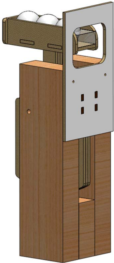
Figure 2: Ammo dump tower. The tower is 4.5" wide, and 12" tall with the feel mechanism plunger between 4 and 8" from the ground.
