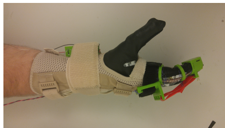
Figure 2.7: Elastic actuation system where elastic will return the finger to its resting position
